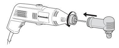
7. Insert the end of the drive shaft into the hole in the right angle attachment.
