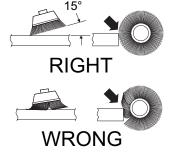
**WARNING** NEVER RUN BRUSHES AT SPEEDS ABOVE 15,000 RPM. The brush could eject bristles at high speed which could become embedded in your skin or which could cause other serious injury.
