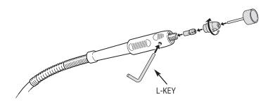
To change the collet or install an accessory in the flexible shaft, follow the same general procedure as for changing the collet and for installing accessories on the rotary tool. To lock the spindle, rotate the collet until the hole in the shaft is aligned with the hole in the flexible collar. Insert the L-key through the holes to lock the shaft.
