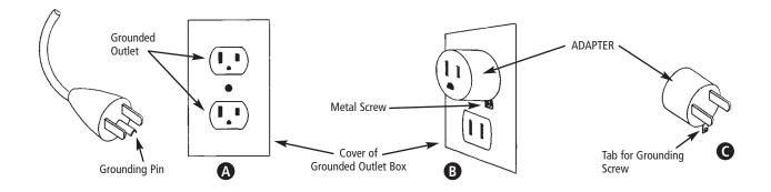
Figure 1 Grounding Method
